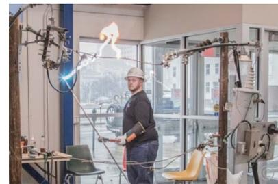
Dayton Power and Light demonstration of electrical hazards near power lines.
